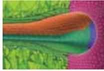
*Multi-zone meshing combines the strength of various meshing tools to automatically generate a hybrid grid for a tidal turbine.*
