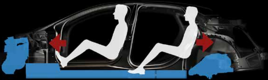
▲ Using a sculpted battery pack allowed for a roomier interior.
