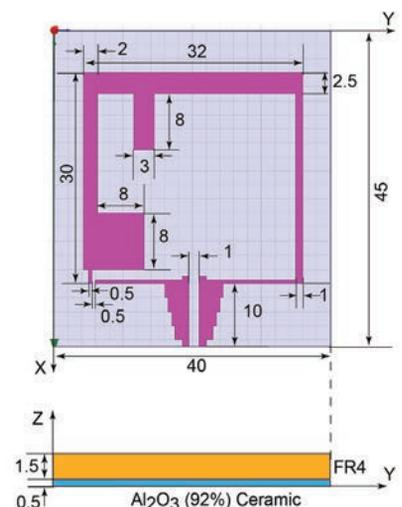
▲ Model of the antenna for an implantable device
