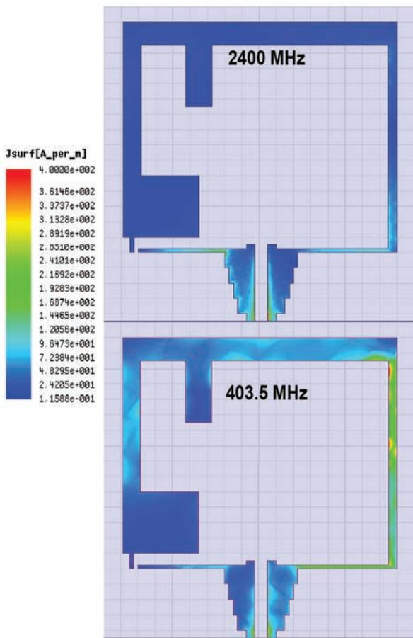
▲ Surface current density for 2.4 GHz and 403.5 MHz, two of the bands in which the antenna must operate
