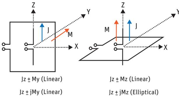
▲ Cambridge Consultants developed a compound field antenna that uses both magnetic loop radiators and co-located electric field radiators.
