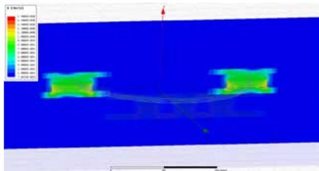
▲ Dynamic 3-D magnetic field simulation with ANSYS Maxwell allowed engineers to determine plate thickness, type of magnets, material used for plates, thickness of the air gap and size of the magnets for each leaf generator.
