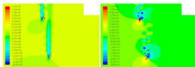
▲ Using fluid dynamics simulation, engineers were able to determine placement of the leaves on the tree so that the wake of one did not affect the next leaf and more power could be generated. Simulations show little effect from wind speed (left) but significant interaction from static pressure (right).
