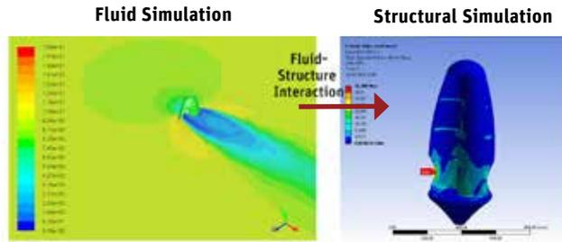
▲ The structure of the ABS wind turbine was examined using fluid–structure interaction.
