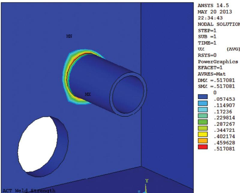
▲ Stresses averaged along a length four times thickness
