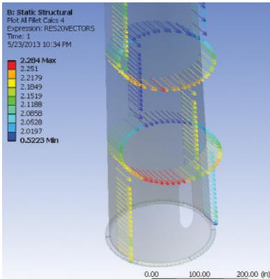
▲ Cost savings achieved on wind tunnel tower by using PJP welds; blue vectors indicate potential PJP welds.
