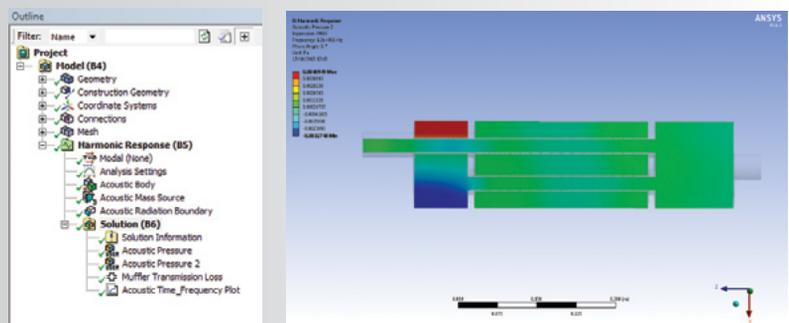
▲ The ACT acoustics extension facilitates performing vibro-acoustics modeling with ANSYS Mechanical software. This extension expedites defining acoustic properties, applying acoustic boundary conditions and loads, and performing post-processing results. An example of a muffler is shown.
