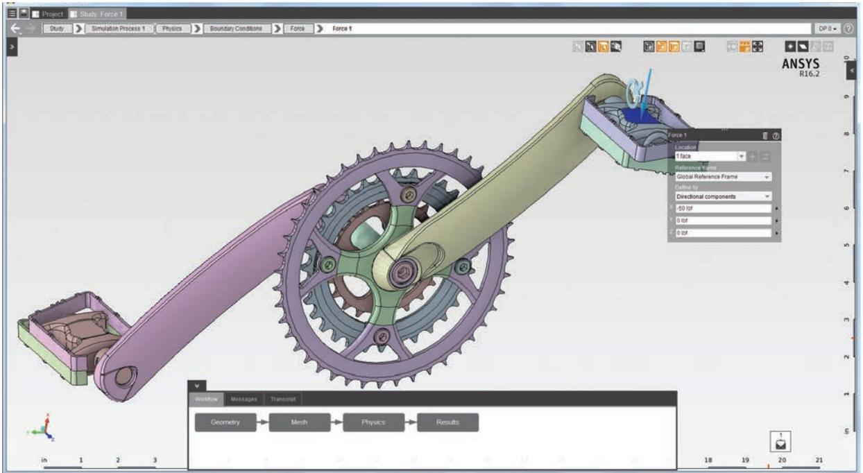
▲ ANSYS AIM's task-based workflow guides the simulation process for static analysis of a bicycle crank assembly. Immersive menus enable quick specification and editing of model inputs and results.
