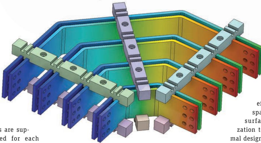
▲ DC electric conduction simulation of a busbar; electric potential shown.
