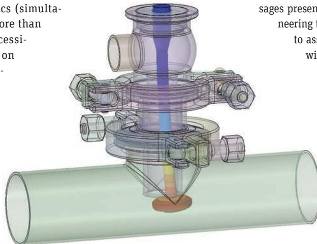
▲ Fluid-structure interaction simulation of a flow control valve. Deformation of the valve stem from fluid forces is shown.
