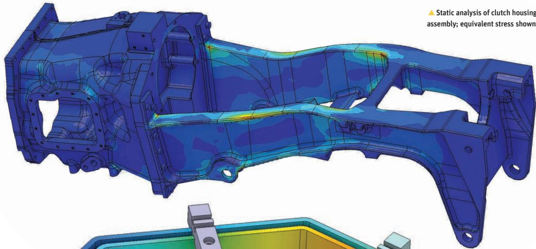
▲ Static analysis of clutch housing and frame assembly; equivalent stress shown.
