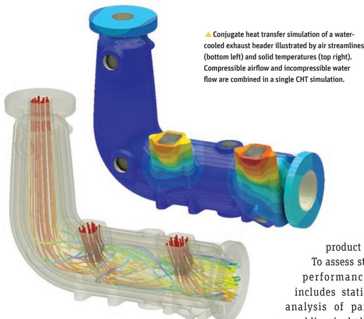
▲ Conjugate heat transfer simulation of a water-cooled exhaust header illustrated by air streamlines (bottom left) and solid temperatures (top right). Compressible airflow and incompressible water flow are combined in a single CHT simulation.
