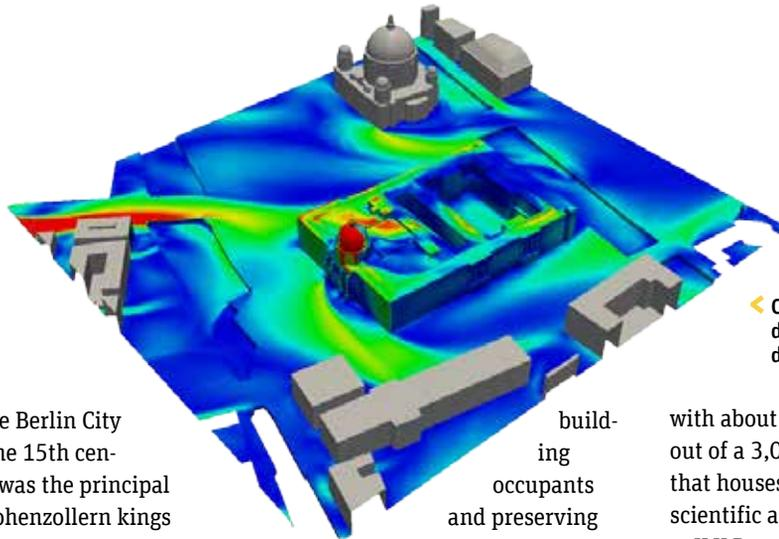
◀ CFD simulation results display pressure distribution due to wind load.
