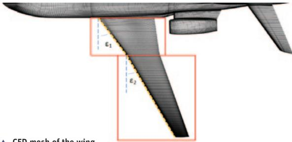
▲ CFD mesh of the wing shows two key design parameters: sweep angles of the two wing parts.
