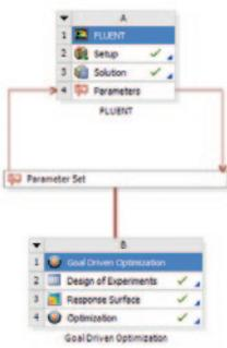
▲ The automation platform triggered the morpher to morph the shape of the wing and to solve the new shape, then passed the results to ANSYS DesignXplorer.
