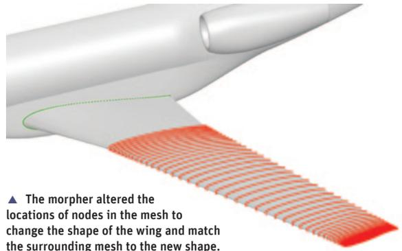
▲ The morpher altered the locations of nodes in the mesh to change the shape of the wing and match the surrounding mesh to the new shape.
