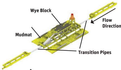
Figure 1. Inline sled structure
