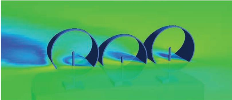
▲ Air velocity with air flowing at 30-degree angle (from right) into original design. Recirculation puts considerable strain on wind turbine at left.
