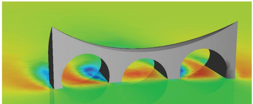
Air velocity with air flowing straight into revised design. There is less recirculation, and wind moves at higher speed through the opening; therefore, this design can extract more energy.
