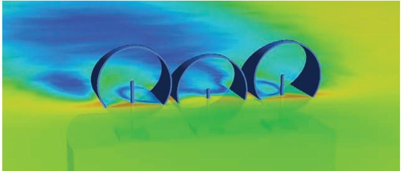
Air velocity with air flowing straight into original design. Low-speed areas shown in blue represent recirculation.
