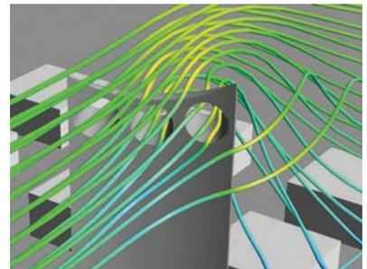
▲ The team created blocks to represent other buildings so that airflow for the turbines could be determined as part of a system. ANSYS software's ability to efficiently handle large differences in scale was important, as the computational domain extended for several kilometers.
