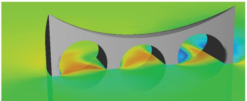
Air velocity with wind flowing at 30-degree angle (from left) into revised design. There is some recirculation in one tube; however, it is considerably less than in the original design.
