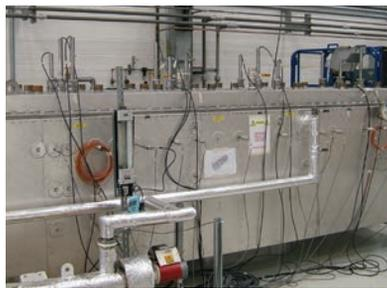
Airbus fuel inerting test rig
