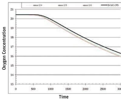
Fluid flow simulation results of the changing oxygen concentration over time (black line) showed consistent close agreement with experimental data taken from multiple oxygen sensors placed inside the inerting test rig.
