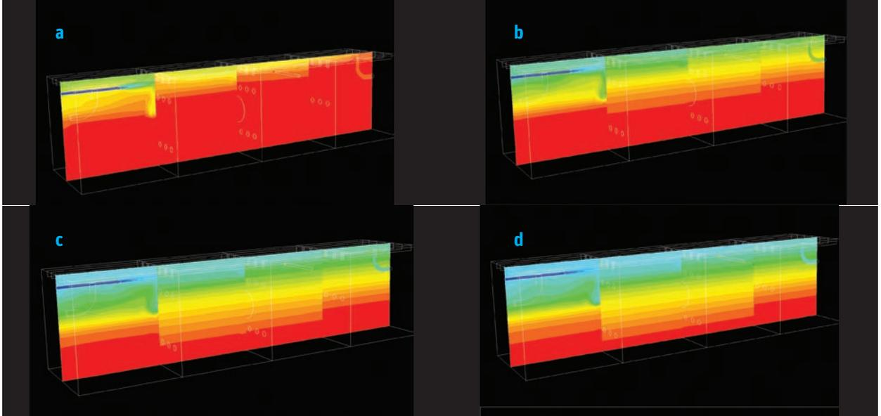
Contours of oxygen volume fraction on a center plane cut of a fuel inerting test rig under simulated cruising conditions at time equal to (a) 4 minutes, (b) 20 minutes, (c) 38 minutes, (d) 50 minutes. Nitrogen gas is injected at the upper left and gradually displaces the air in the rig's four compartment bays; the gas is then vented through an exhaust opening at the upper right.
