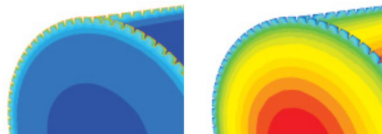
Close-up view of contours inside a microfin tube, temperature (left) and velocity (right)
