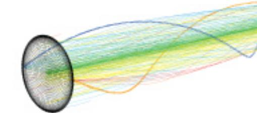
Pathlines of the particle flow inside the microfin tube colored by particle ID
