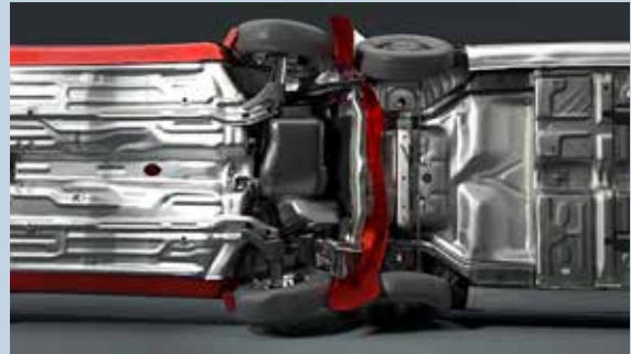
Viewing a rendered LS-DYNA crash simulation from below. Rendering courtesy of Ed Helwig.
