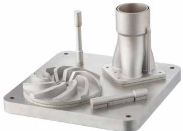
Additive manufactured parts with specimens for mechanical testing on a build plate are shown here.
