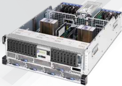
A 4U IBM Power System Server with the cover off
