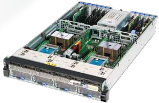
A 2U IBM Power System Server with the cover off
