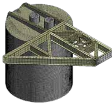
Finite element mesh of a suction pile
