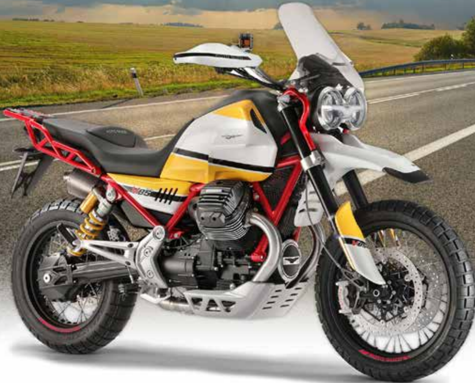
The Moto Guzzi V85 is equipped with an 80 HP twin cylinder engine.
