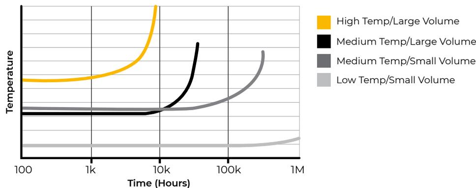
There are several things that a designer can do to mitigate the higher temperature effects on magnetics. For example, the device could utilize a low loss core material. Also, higher frequency with total turns reduction while maintaining turns ratio or using Litz wire for reduced coil heating can be done. Or, varnish applied with vacuum evacuation (also allows for washing) can also facilitate improved thermal performance.
