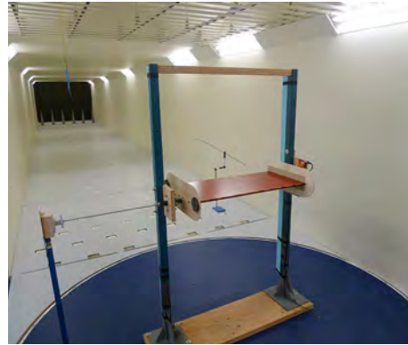
Model used for wind tunnel testing
