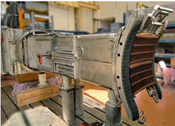
Plasma current drive antenna in isolation Courtesy: C. Roux, R. Volpe, CEA
