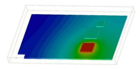
HyperSat electronics board thermal analysis results (Ansvs Icepak)
