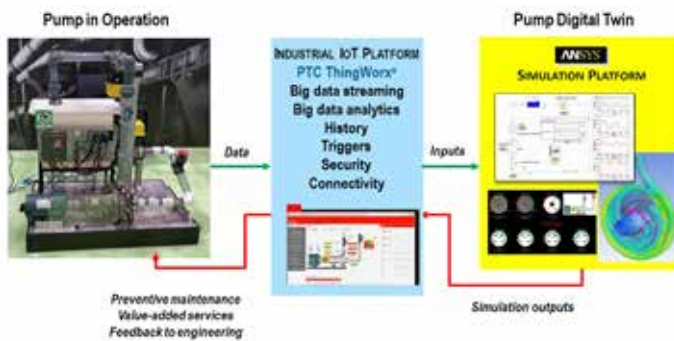
▲ The real pump connects to its digital twin using ThingWorx.
