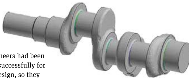
▲ Crankshaft fatigue analysis using ANSYS nCode DesignLife
