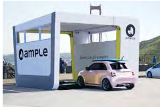
Ample single port battery swapping station
