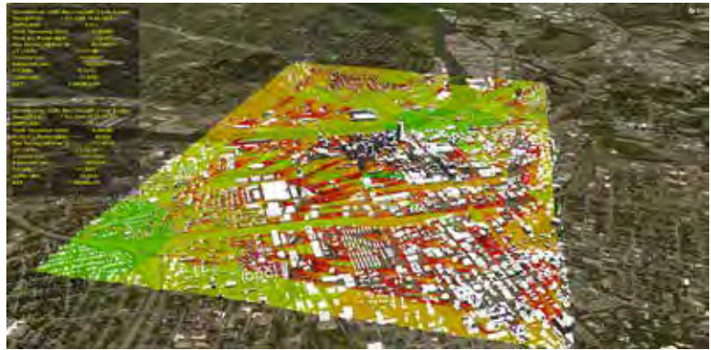
A commercial unmanned aerial system operation being modeled within an urban environment. Data like the expected signal quality shown at mission altitude from available cellular network stations would be useful for autonomous vehicles in smart cities.
