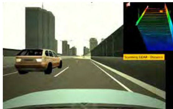
A simulated lidar sensor image produced by Ansys AVXcelerate
