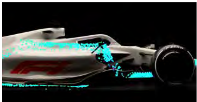
Ansys Fluent simulation showing air flow under and over the Formula One race car chassis
