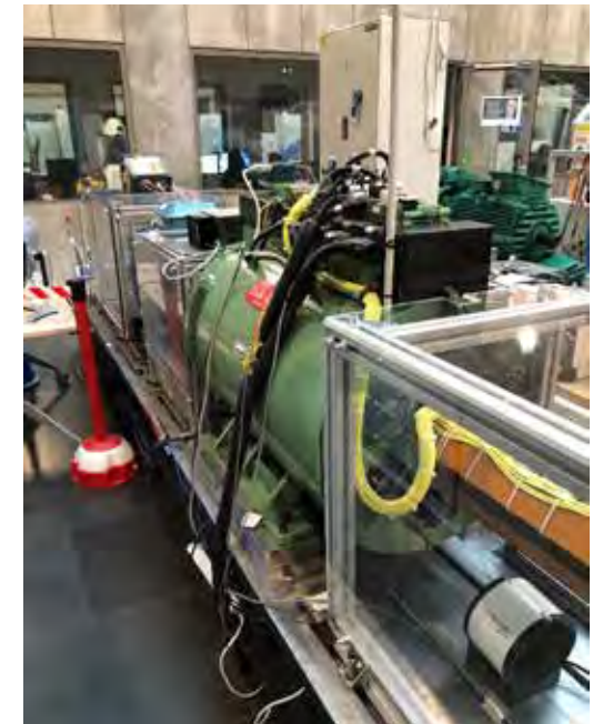
ConnexITy’s turbo generator test bench, located at the ConnexLab on the Saclay plateau in Paris, France
