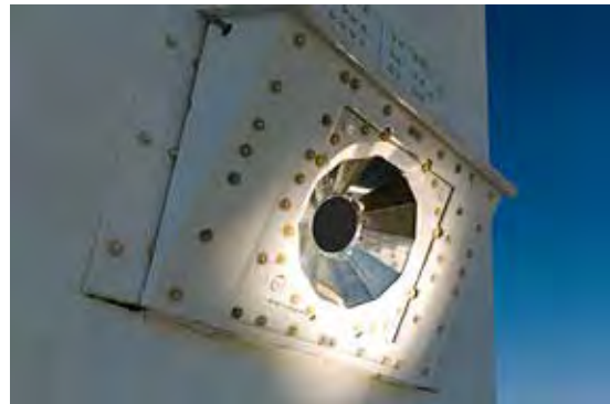
Closeup of Synhelion’s proprietary solar receiver, which provides the necessary process heat to produce solar fuels. Image courtesy of Synhelion.
