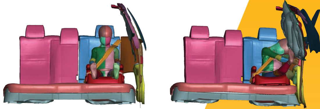
Simulation of a child passenger in a car seat before a side impact collision (left) and during collision
