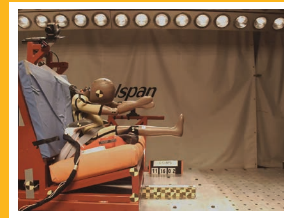
Physical testing using a crash dummy to verify simulation results
