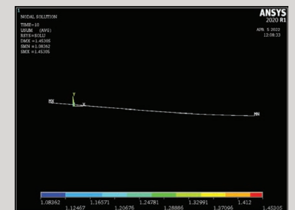
Ansys Mechanical model of the deformation of a 3-km natural gas pipeline subjected to multi-support excitation, simulating the effect of an earthquake for 10 seconds
