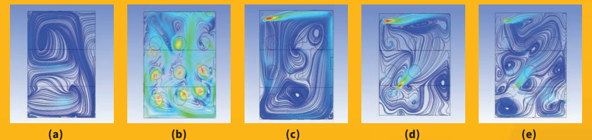
Velocity streamline contours for (a) baseline case simulation, (b) simulation with ceiling fans and an exhaust fan switched on, (c) simulation with one exhaust fan and one pedestal fan, (d) simulation with one exhaust fan and two pedestal fans, and (e) simulation with two exhaust fans and two pedestal fans
