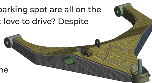
Lower control arm mesh in Ansys Mechanical
