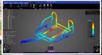
A structural analysis of the AdvenChair frame in Ansys Discovery
