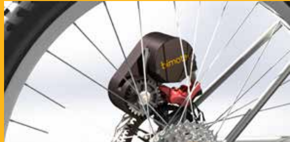
The Bimotal Elevate is a removable, lightweight e-bike motor that mounts to your bike’s disc brakes.
