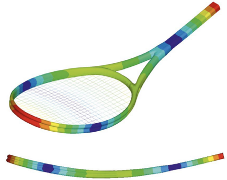
First bending mode of a strung tennis racket in elongation. Hitting the ball at the blue node line on the strings does not excite this mode. This is the sweet spot of the racket.
