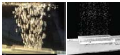
Left: A conventional gas diffuser produces relatively large bubbles. Right: A gas diffuser with the fluid oscillator shows tremendous reduction in bubble size.
