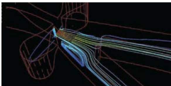
Pathlines later in the cycle showing that flow through the control nozzles has overcome internal feedback and the main jet is being switched to the lower outlet channel
