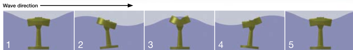
COLUMBIA POWER's wave power system: The wings and vertical spar react to the shape of the passing ocean swell. Each wing is coupled by a drive shaft to turn its own rotary generator.
