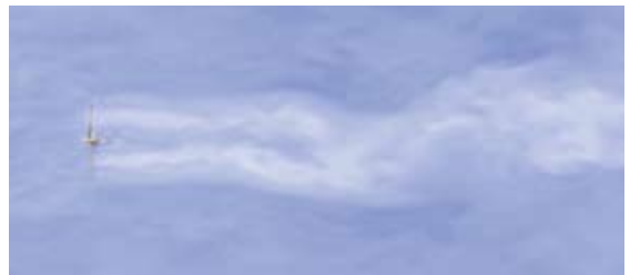
Meandering wake behind an ENERCON E-66 wind turbine. Blue represents high wind speed, and white represents low speed.
