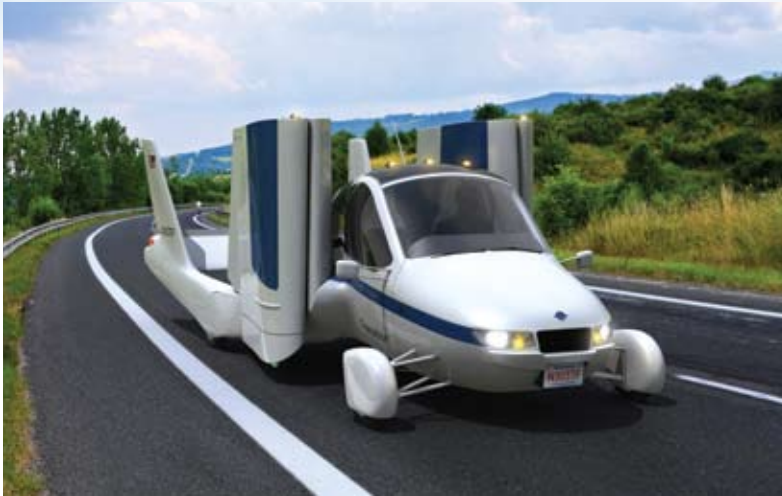
The Transition's foldable wings allow the aircraft to be driven on the highway as well as parked in a typical residential garage.
