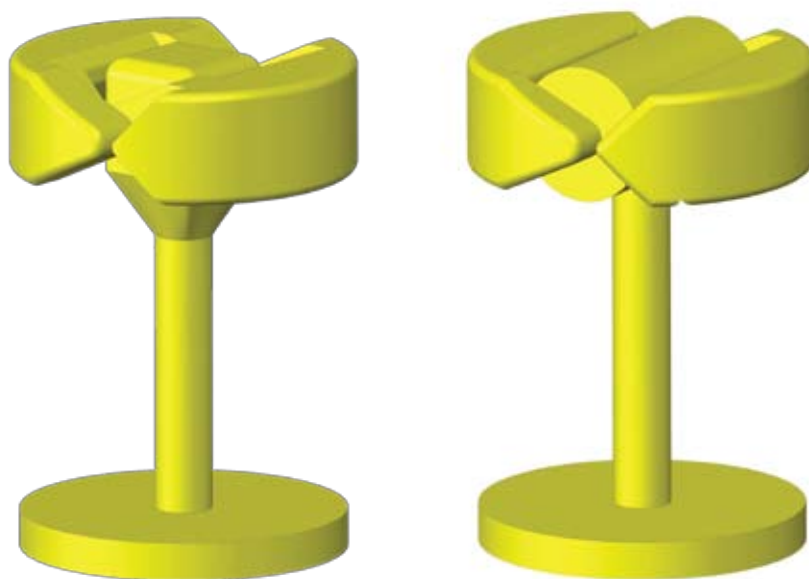
COLUMBIA POWER engineers doubled efficiency of the buoy by using ANSYS AQWA to optimize its geometry.
