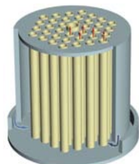
Configuration of a 36-tube anode-supported SOFC stack
