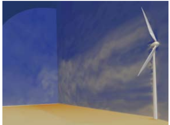
Wind field behind an ENERCON E-66 wind turbine with hub height of 65 meters. The blue color indicates high wind speeds, and white indicates low speeds.
