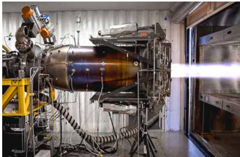
Hermeus' proprietary turbine-based combined cycle (TBCC) engine, Chimera, is a hybrid turbojet-ramjet engine capable of powering hypersonic aircraft at Mach 5 speeds.
