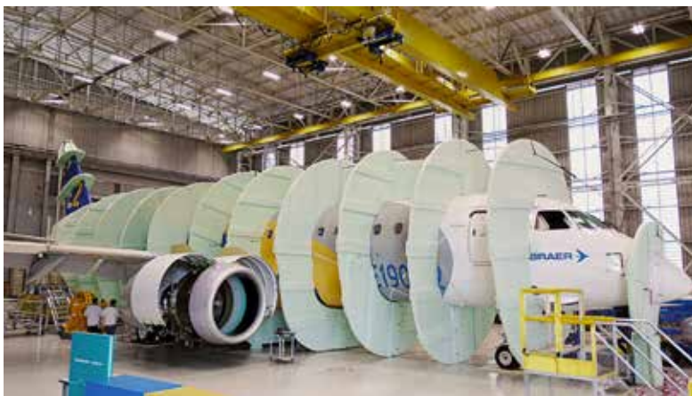
During physical testing, electrical discharges are created in a structure enveloping the aircraft. Induced current passing through a critical component’s harness is measured to evaluate the effects of lightning strikes. Image courtesy of Embraer.
