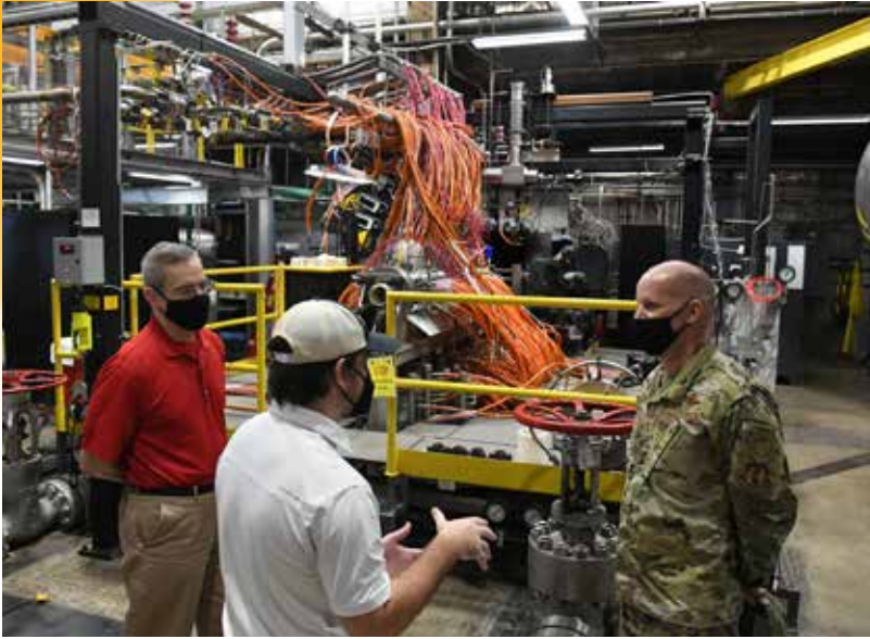
John Hile, center, an Arnold Engineering Development Complex (AEDC) test engineer, speaks with Maj. Gen. Evan Dertien, commander, Air Force Test Center, about the use of arc heaters, such as the one seen in the background, for characterizing and evaluating thermal protection systems. Also pictured is Frank Wonder, arcs capability manager. U.S. Air Force photo by Jill Pickett
