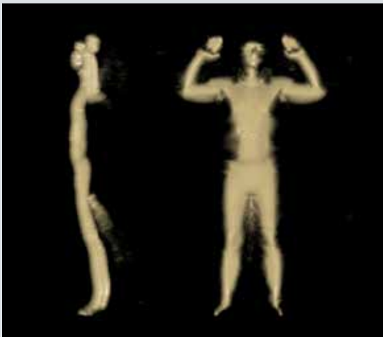
Use of 5 GHz bandwidth and 60-degree beamwidth showed impact of reduced depth resolution on image quality.
