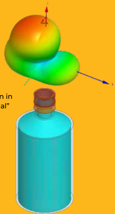
The 3D radiation pattern of the dipole antenna when it is mounted on top of the bottle
