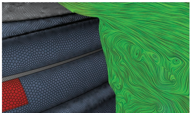
Mosaic-enabled mesh was used to capture details of turbulent flow around the rear of this car.
