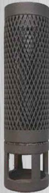
First attempt to produce the part by additive manufacturing resulted in considerable distortion.
