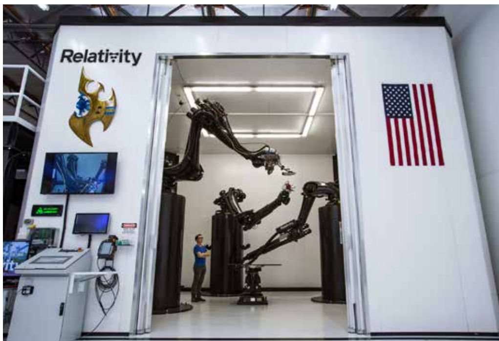
Measuring 15 feet tall and nine feet in diameter, Relativity's Stargate is the world's largest 3D printer. The startup is currently using ANSYS Additive Suite to optimize the printer's performance.
