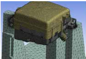
FEA model for vibration fatigue simulation
