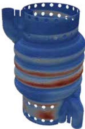
ANSYS Additive Print predicts displacement for a heat exchanger. Courtesy Additive Industries.
