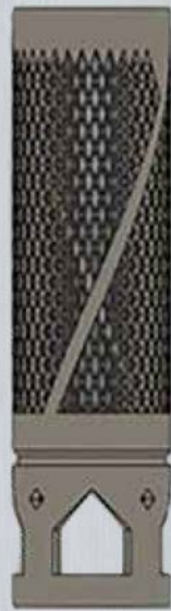
CAD model of redesigned part with supports incorporated into mesh
